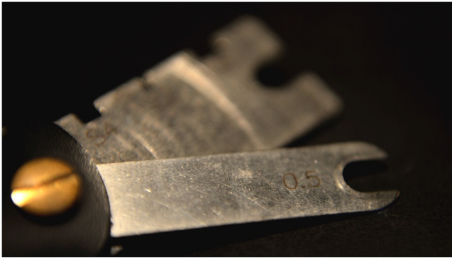
Shims to test the travel of épée tips.
